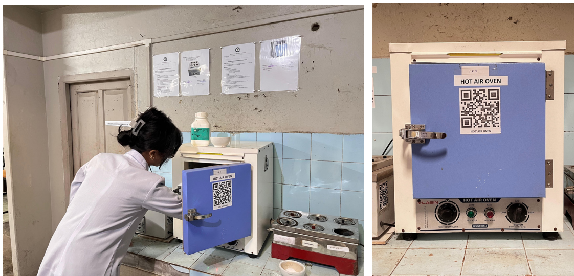
Fig. Determination of Moisture Content using hot air oven
